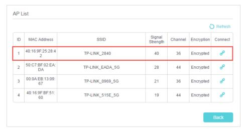
5. Click the connect icon and then the SSID and MAC will be automatically filled in. Configure the Security settings as the AP you choose to be bridged.
