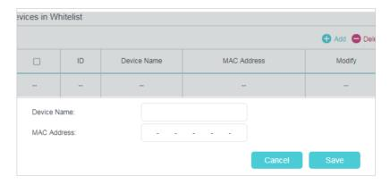
3) Enter the Device Name and MAC Address (You can copy and paste the information from Devices Online table if the device is connected to your network).
